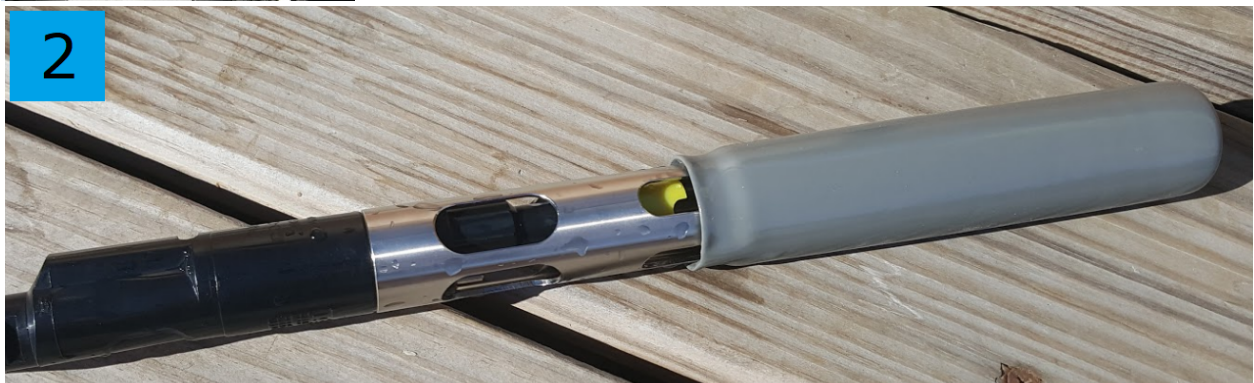
Figure 2. Remove sleeve from sensor guard. Submerge the sensor in the upweller at the end near the outfall pipe (Harold's work shed side). Let it sit for a few minutes.
