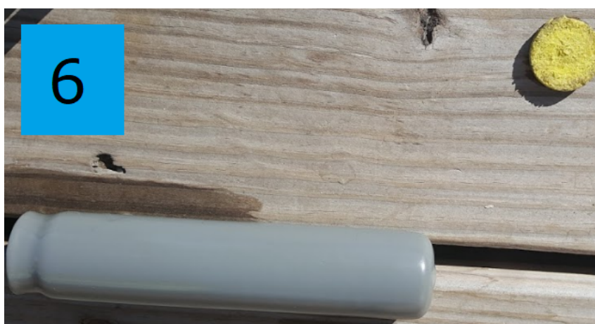
Figure 6. Check to make sure the little sponge in the sensor guard is moist. Replace the sponge and put the sensor guard back on the sensors.
