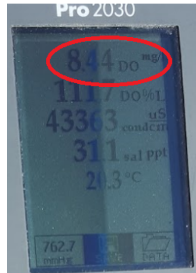
Figure 3. Once the sensor has sat in the water for a few minutes, jig it up and down in the water column. You will see that the top number (DO mg/L) will change. Continue jiggling, keeping the sensor submerged until the number holds steady. That is the value you use for the DO on the data sheet.
